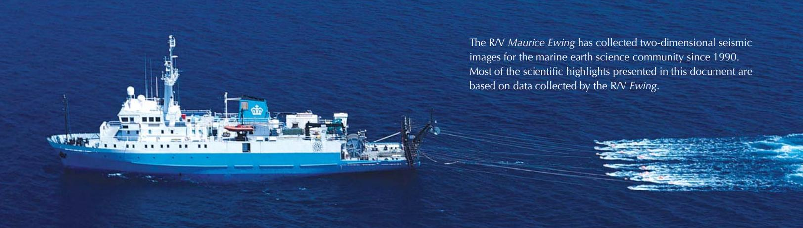
The R/V *Maurice Ewing* has collected two-dimensional seismic images for the marine earth science community since 1990. Most of the scientific highlights presented in this document are based on data collected by the R/V *Ewing*.
