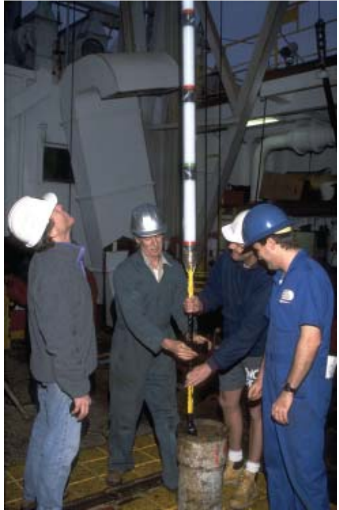
Figure 12. Earl Davis, Keir Becker, Geoff Wheat, and Bill Rhinehart attaching OsmoSampler to bottom of cable during initial stages of deployment on ODP Leg 168 (Juan de Fuca Ridge). The OsmoSampler was deployed for three years. Upon recovery, the sampler yielded weekly fluid samples, thus providing a unique time-series of the chemical composition of formation fluids in an open borehole. These data are used to assess the rate of seawater flow within the upper permeable basaltic basement and to constrain the composition of formation fluids. Determining the composition of these fluids has been a long-term goal of DSDP and ODP and is critical to our understanding of crustal alteration and evolution. An amazing result from this work is that even after three years, the hydrologic system has not recovered from drilling operations. Photo courtesy of Keir Becker, University of Miami.
