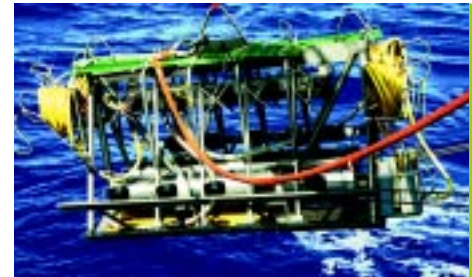
In September 1998, a permanent, deep-ocean scientific research facility—the Hawaii-2 Observatory, or H2O—was installed on a retired AT&T submarine telephone cable that runs between Oahu, Hawaii and the California coast. Shown here is the seafloor junction box being deployed from the R/V Thompson . Photo courtesy of F. Duennebier.
