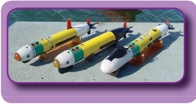
Figure 5. REMUS AUVs configured with forward-looking, high-resolution sonar, a sidescan sonar, acoustic communication, and various other environmental sensors. AUVs such as these have proven especially useful in coastal surveys of bathymetry, currents, and water properties. Photo courtesy of Chris von Alt, Woods Hole Oceanographic Institution.
