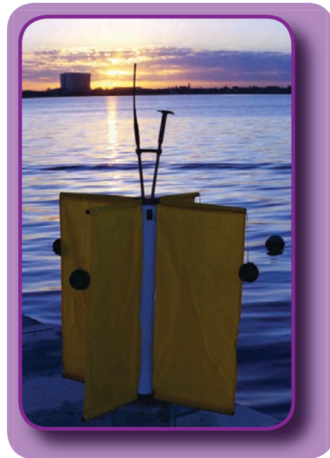
Figure 2. Coastal Ocean Dynamics Experiment (CODE) drifters follow the top meter of the surface ocean, where they respond to the instantaneous wind forcing. The small ball floats help keep the drifter upright and the currents push the “X” shape through the water. The GPS receiver and satellite transmitter antennas are sticking up from the top of the drifter. From http://www.ims.uaf.edu/NPRBdrifters/planview/code.html , courtesy of Technocean, Inc.
