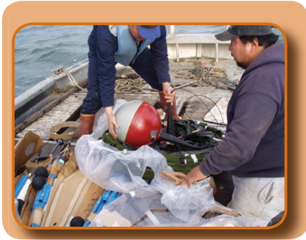
Figure 1. Preparing to deploy a Surface Velocity Programme (SVP) drifter in the Bering Sea. One of the goals of this drifter program was to demonstrate that drifters could be economically deployed by lay persons, in this case by villagers in a remote Alaskan community. SVP drifters move with the current at 10 m depth. From http://www.ims.uaf.edu:8000/NPRBdrifters . Photo by Larson King.
